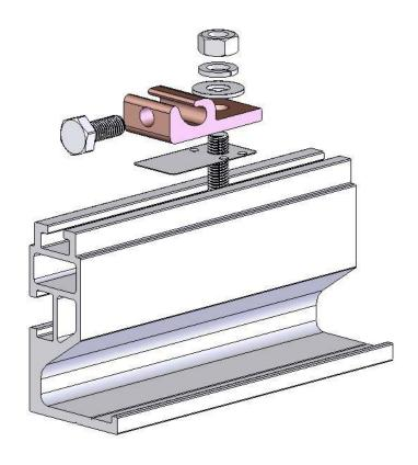
Figure 2. WEEBLug mounted on rail.
