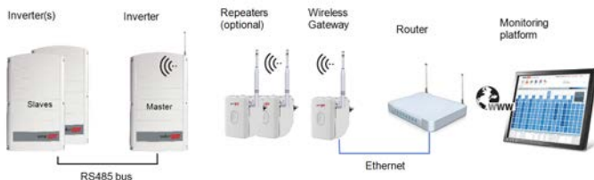
Figure 3: Multiple inverters, wired connection
