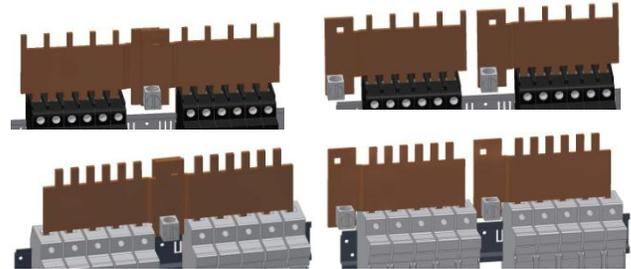
The **MNPV12-250** comes with 168 amp busbars that work with up to six of the MidNite 300VDC breakers. The MNPV12-250 busbars may be joined to accommodate 6 strings or separated for two independent sets of three strings.
