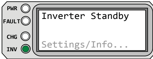
Figure 5-6, Inverter Standby Mode
